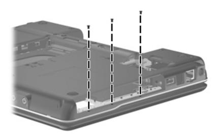
Where used: 3 screws (in optical drive bay) that secure the top cover to the computer
